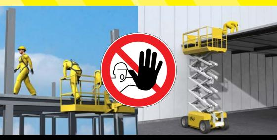
Mobile elevating work platforms (MEWPs) are specifically designed to lift people to a position where they can work at height safely within the platform.
